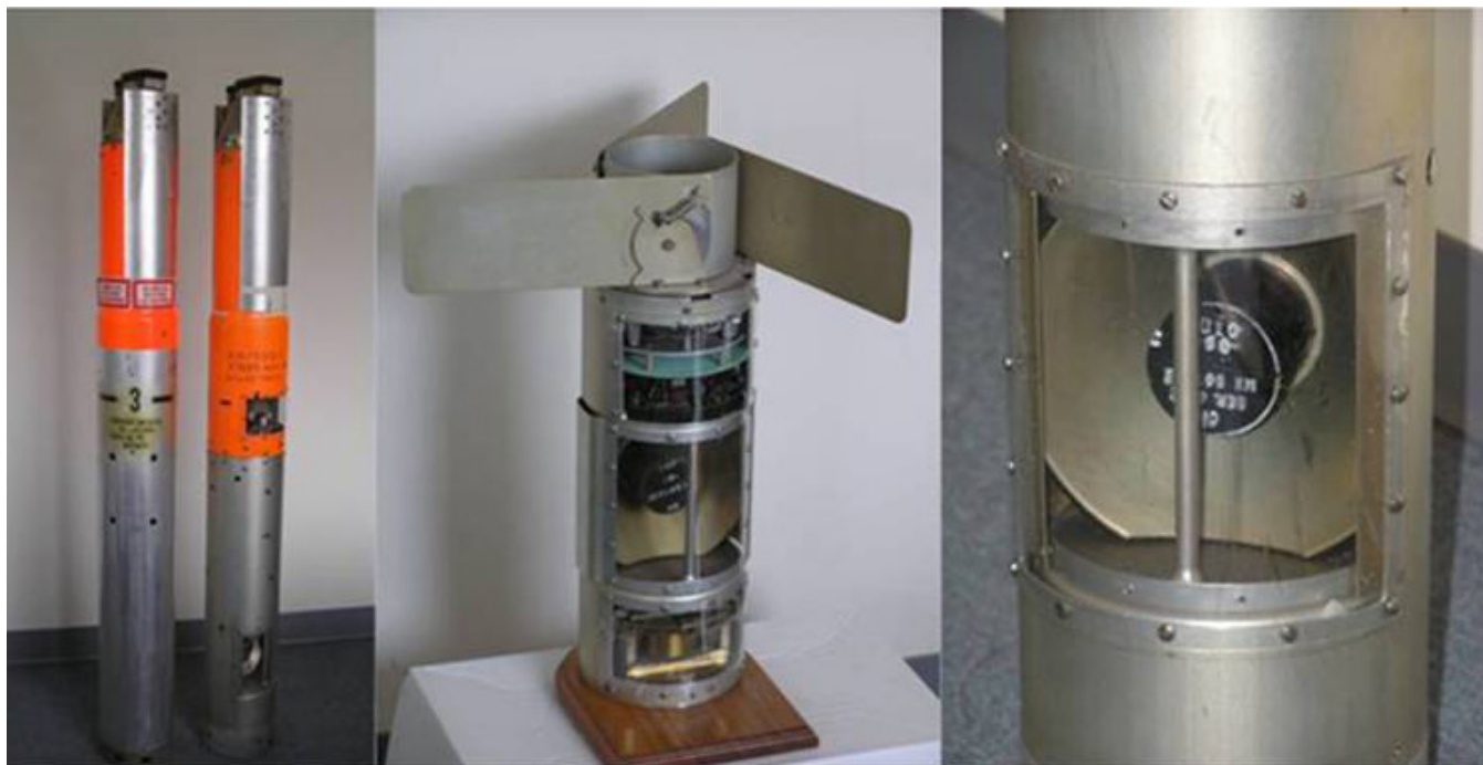
Fig. 7 – AN/SSQ-1 and 1A Sonobuoys Showing the Rotating Directional Hydrophone
